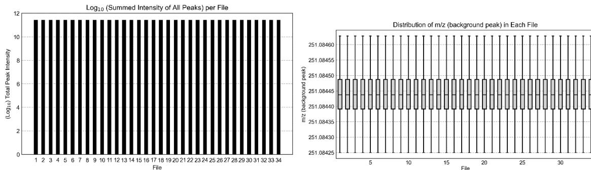
m/z 242.0175 was selected as background peak to check the mass accuracy for 34 samples in carboxyl channel analysis. The summed intensity of all peaks was consistent during all runs. The mass of the background peak was consistent during all runs and all are within the expected range, showing good stability and mass accuracy for data acquisition.
